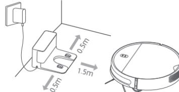
Note: Make sure the charging dock is in a well-lit environment without direct sunlight. Clear off the reflective objects such as mirrors nearby to avoid affecting the returning back of the vacuum-mop to the charging dock. Do not place the charging dock on the table to prevent it from falling down.
