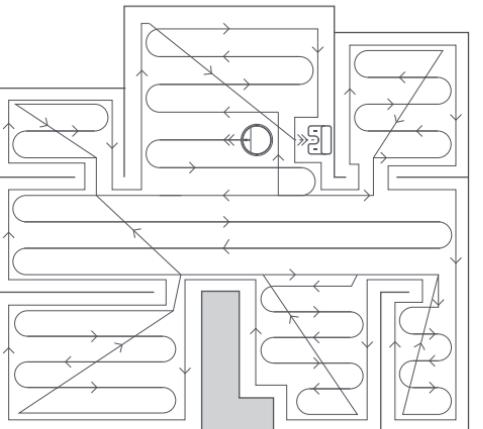
\* During a cleaning task, the vacuum-mop enters and exits the rooms, and confirms the boundary of the room and furniture by touching it. This is normal and does not affect the cleaning efficiency.
