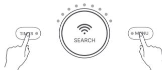
If the device cannot connect to your phone, press the "MENU" and the "TIMER" buttons simultaneously for 5 secs to reset. The yellow indicator light will blink to show that Wi-Fi has been reset successfully and you can reconnect to the network.
